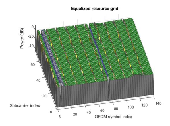
As can be seen the equalization flattened the power response across the resource grid.
